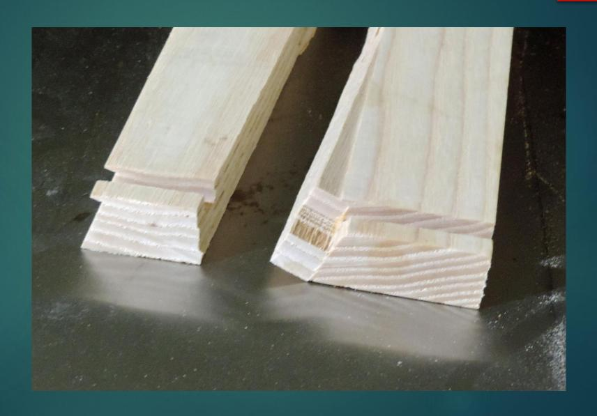
Do a dry fit to make sure all the joints are tight and the disc fits.
